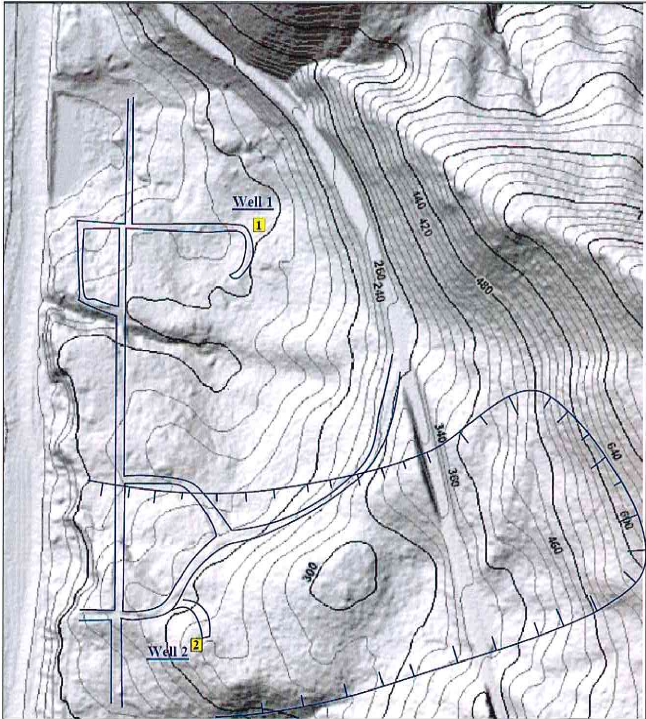
Figure 2: LIDAR shaded relief topographic map for the north part of Cove Beach. Well 2 lies within a rubble flow deposit consisting mostly of sandstone. Well 1 is in rubble flow of mudstone and sandstone. These mass wasting deposits are estimated to be perhaps more than 10,000 years old and are suspected of being triggered by a combination of both seismicity and Ice Age weather conditions.
