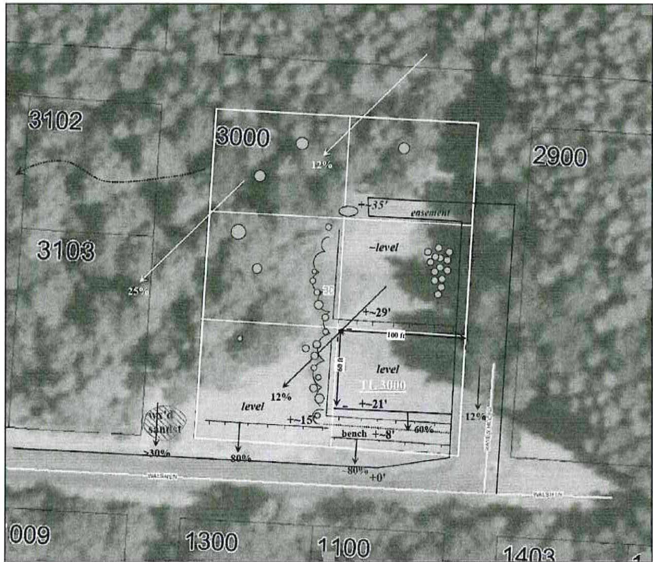
Figure 4: Site-specific observations for TL 3000 and nearby lots. Spheroidally weathered basaltic boulders are shown stacked west and north of the property. The proposed house should be constructed at least 10 ft back from the steep break-in-slope in the southern one-third of TL 3000, away from the embankment above Walsh Lane. The original slope for this property is estimated to have been about 12 percent to the southwest. The height of the leveled area is roughly 13 ft above the base of the upper cut bank, which is inclined from 50 to 80 percent. Given the presence of weathered sandstone exposed in Third Avenue in the partially excavated road cut west of the property, the cut bank can be expected to support a 1.5H:1.0V slope. It would be prudent to keep all foundations at least 10 ft back from the top of the cut. The bearing capacity of the gravelly clay-silt soils will be no less than 1500 psf. There may be hidden blocks of basaltic breccia buried beneath the surface of the lot, but it will disaggregate with a chisel-tipped rock breaker mounted on an excavator. Mapping after Horning (2013).
