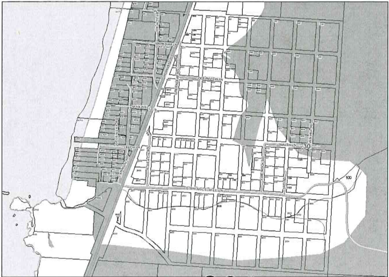
Figure 2: Geologic landslide hazard overlay (orange) for the southern part of Arch Cape. Tax Lot 3000 lies just within the area considered to be old landslide, on the northwest corner of the intersection of Walsh Lane and Raven Hill Road.
